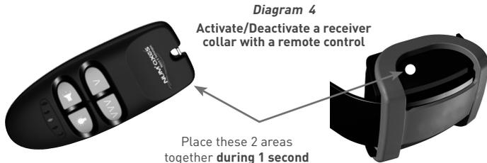
◆ **Coding of the remote control and receiver collar**
